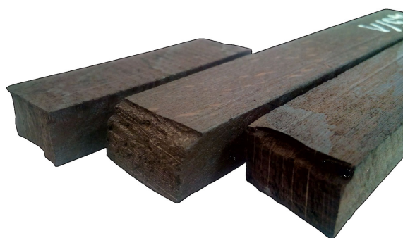
Figure 8. Typical brittle fracture patterns of fixated and thermally modified specimens at 200 °C.
