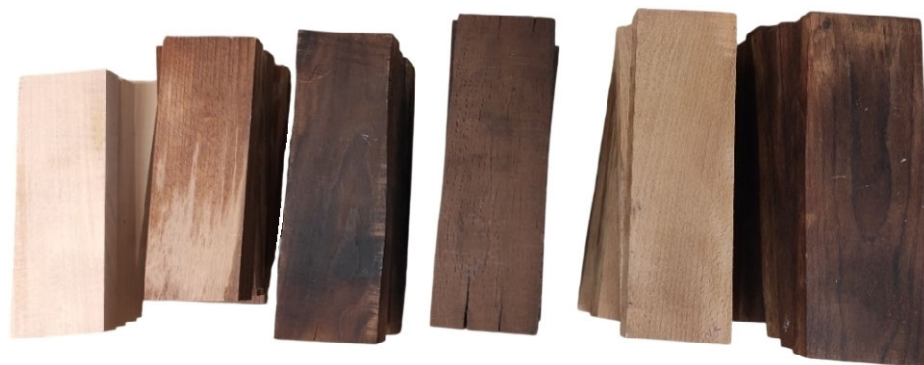
Figure 1. Ready lamellae of the six samples (from left to right: Untreated; Impregnated 120 °C; Impregnated 160 °C; Impregnated 120 °C and Thermally treated; Thermally treated; Thermally treated and Impregnated 120 °C). Thermal modification was performed at 180 °C. Impregnation was carried out using oligomeric lactic acid, followed by polymerization at the temperatures indicated for each sample.
