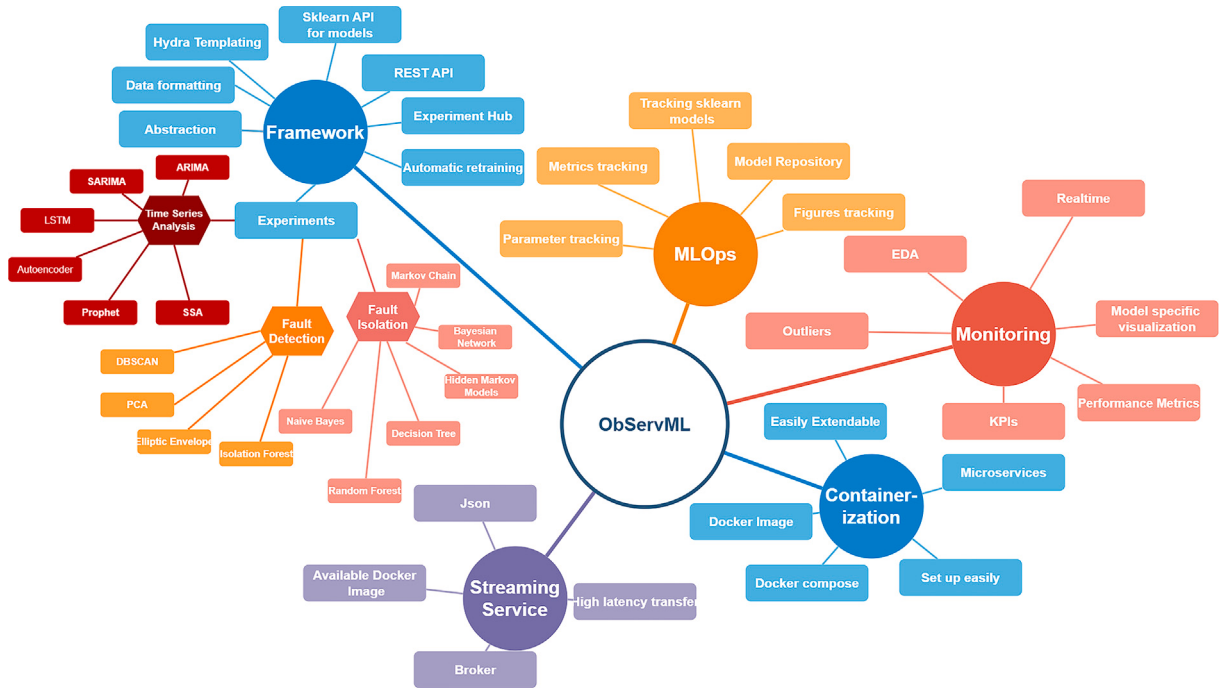
Fig. 1. Concept map of the developed ObServML python package. The colored circles denote the microservices, whilst rectangles present a feature of the service. For the Experiments features, more concrete information is depicted in forms of the problems it can solve (fault detection, fault isolation and time series analysis). Process mining is not on the concept map as it is only an experimental feature.
