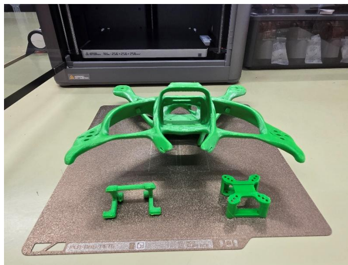
Figure 2: Drone parts made with a Bambulab X1E 3D printer
