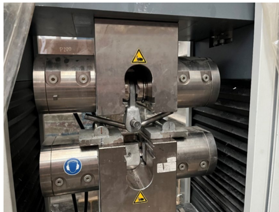
Fig. 6. Set-up for three-point bending tests.
