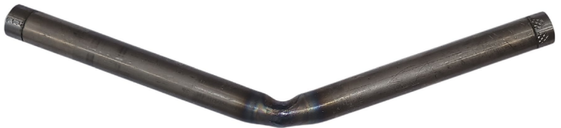
Fig. 13. Deformed shape of a butt-welded joint subject to three-point bending test.
