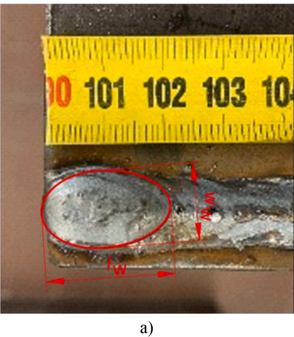
Fig. 7. a) Weld pool length and width; b) evaluated aspect ratios plotted against Rosenthal numbers (indicated by red dots) in relation with slow and fast regimes as referred to in [44].
