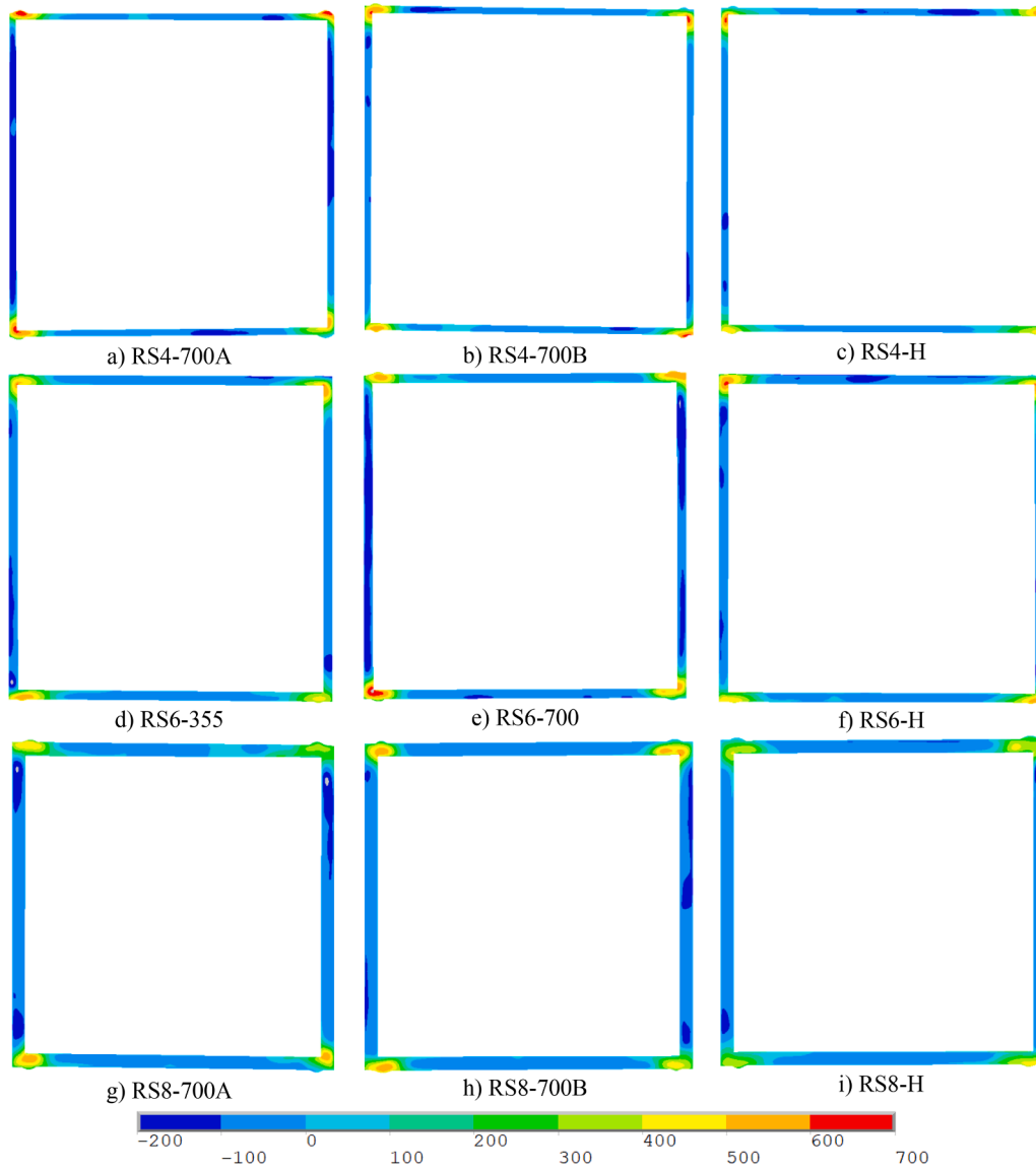
Fig. 20. Longitudinal residual stresses ( \sigma_{rs,z} ) in [MPa] for all nine specimens.
