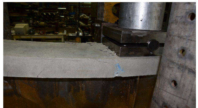
Fig. 14. Upper flange crushing in B1/1.
