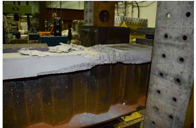
Fig. 22. Upper concrete flange failure (B3) – side view.
