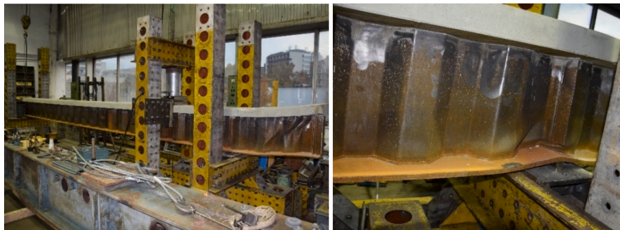
Fig. 16. Deformation of the specimen B1/2.
