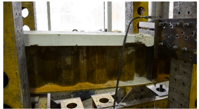
Fig. 28. Crushing of the upper concrete flange of B5/2.
