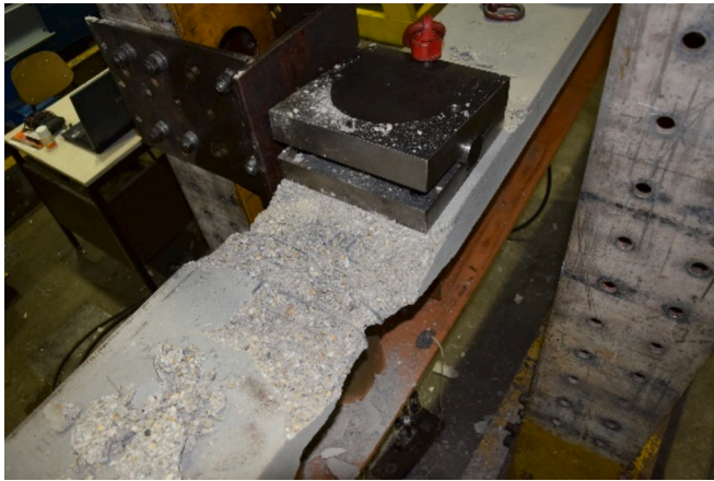
Fig. 26. Concrete flange failure of B4 – view from above.
