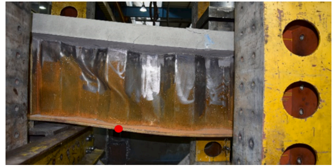
Fig. 13. Shear failure of web in B1/1 (red dot presents inflection point). (For interpretation of the references to colour in this figure legend, the reader is referred to the web version of this article.)
