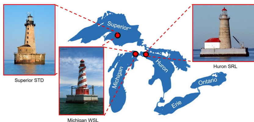
Figure 1. Great Lakes Evaporation Network sites (red dots) with photos of the stations used in the analysis, including Stannard Rock Lighthouse at Lake Superior, White Shoal Lighthouse at Lake Michigan, and Spectacle Reef Lighthouse at Lake Huron. Eddy-covariance and routine weather measurements are carried out at the top of these lighthouses (Blanken et al., 2011; Spence et al., 2011).
