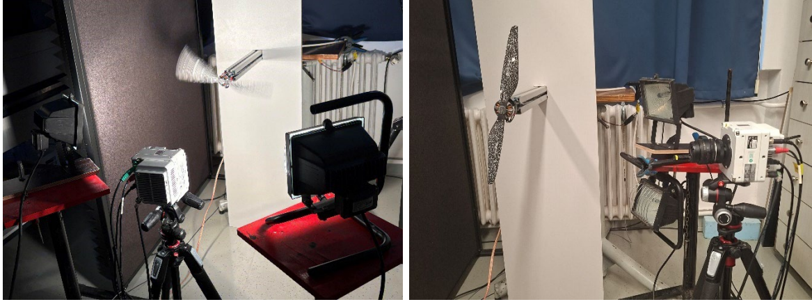
Figure 13: Rotating drone propulsion system high-speed camera measurement setup. (Left side: front view for in-plane motion, Right side: side view for out-of-plane motion)
