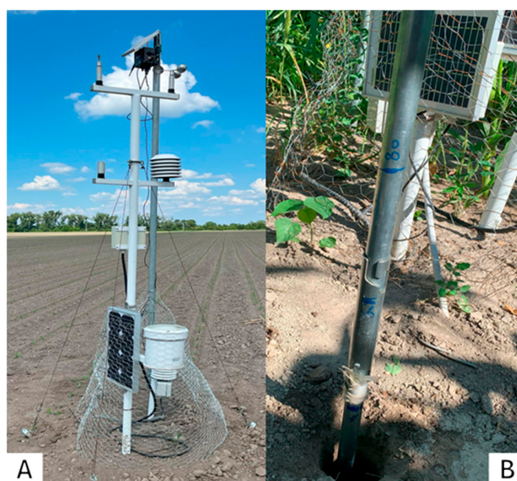
Figure 2. (A) IoT-based meteorological sensor station within the field. (B) Collecting soil samples using a hand auger from sampling points around the sensor stations.
