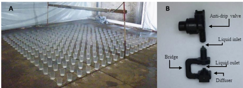
Fig. 2. A: Collectors distributed under the nebulizer for distribution evaluation. B: Tavlit 20 nebulizer. Own creation
