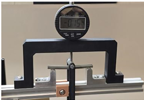
Fig. 3. Bending test set up (Own creation)
