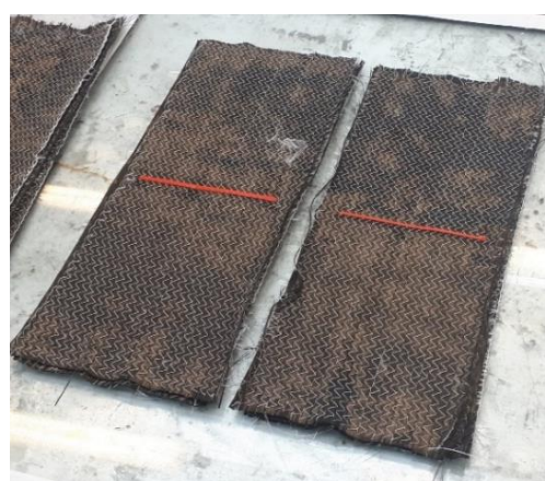
Figure 2. UD carbon fabric containing the PCL interlayer material during the manufacturing of the tensile test specimen.
