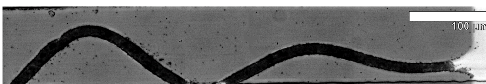
Fig. 14. Fishbone, snake and sine electrodes during operation. The diameter of the collected particles is 1 \mu\text{m} .
