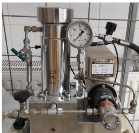
Fig. 3. Photo and schematic drawing of Celfa P-28 test membrane apparatus.
