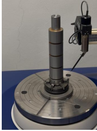
Figure 3. Talyrond measurement setup with vertically mounted machined specimen and contact probe.
