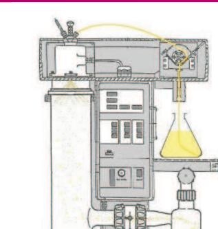
Co-spray-drying procedure: Inlet temperature: 140 °C Feed rate: 005 % Aspirator air: 600 L/min Aspirator rate: 75 %
