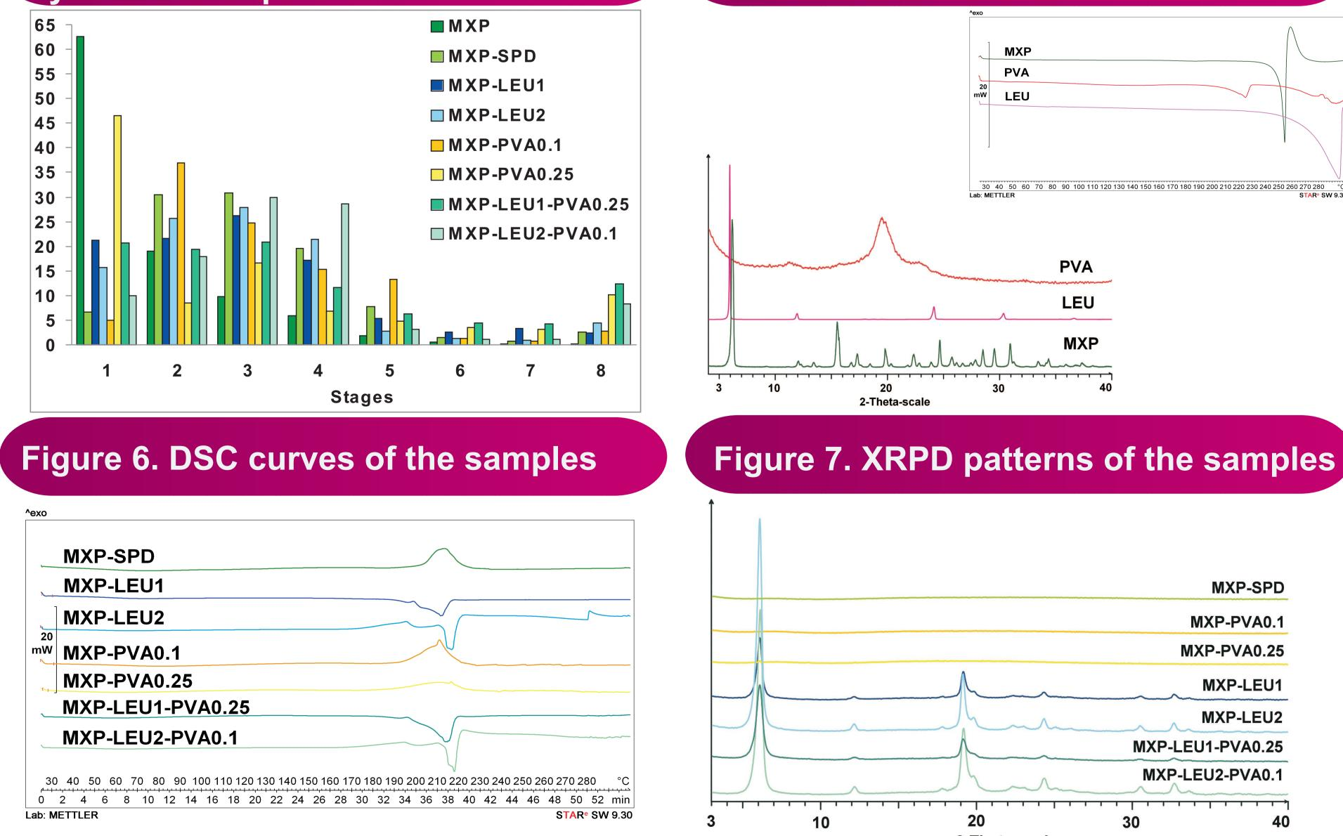
can conclude that the raw MXP is crystalline and additives are semi-crystalline materials. The crystalline form of MXP turned to amorphous character in the presence of PVA (crystallization inhibitor effect). When LEU was applied the characteristic peaks of MXP on the XRPD patterns and its melting on the DSC curves were detected (Figs. 5-7).
