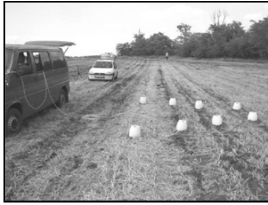
Figure 9. The test car and the portable chambers
