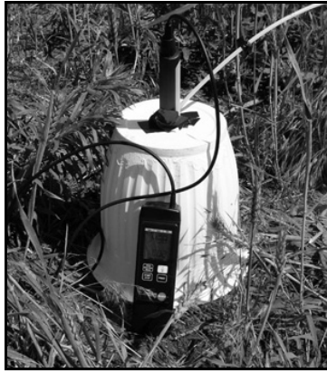
Figure 8. TESTO 535 CO 2 tester and portable chamber
